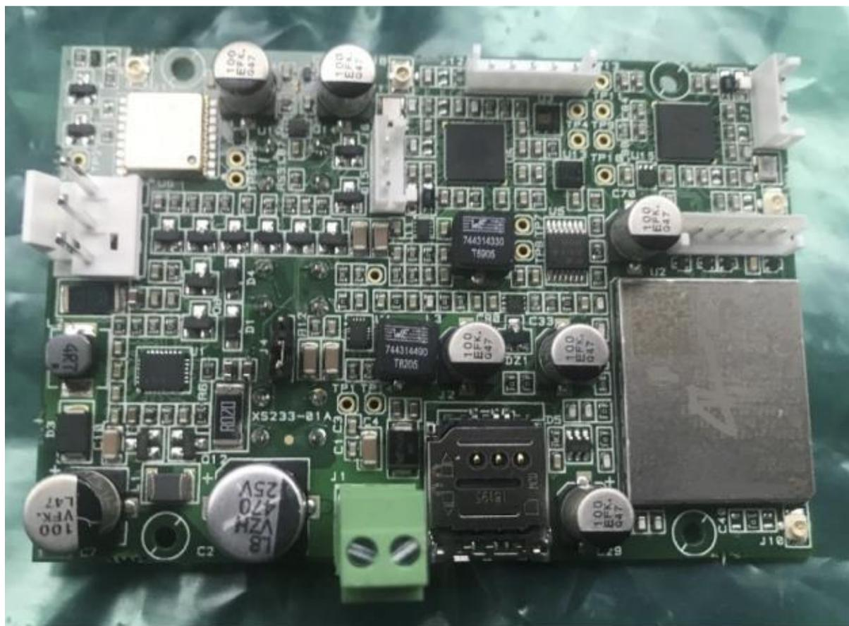
**The Micro-Flexx board, an NGS designed and deployed sensor and tracking device (Image source: NGS).**
